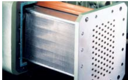
Intercoolers/Aftercoolers – Water-in-tube intercooler and aftercooler bundles slide out for easy inspection and cleaning.
