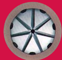
Variable Inlet Guide Vanes – Variable inlet guide vanes can offer power savings of up to 9%. Inlet vanes impart a whirling motion to the inlet air flow in the same direction as the impeller operation, reducing the work input. Net power savings at reduced flow or on days colder than the design temperature. Inlet vanes are positioned close to the impeller to achieve maximum benefit.
